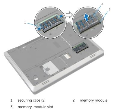
2 Slide the memory module away from the memory-module slot.
