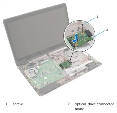
2 Slide and lift the optical-drive connector board away from the computer base.
